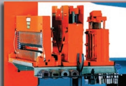
Tool table extension with punch and die storage - 6509, 9012, 12012, DO 70, DO 95, DO 120, DO 135, DO 150
