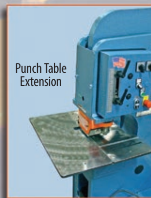
Tool table extension with punch and die storage - 6509, 9012, 12012, DO 70, DO 95, DO 120, DO 135, DO 150
